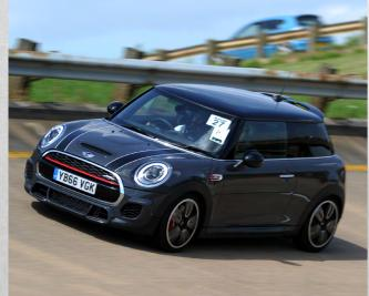
Millbrook's five lane. two mile, banked High Speed Bowl is where realistic motorway driving can be simulated in a safe and secure setting. Test lane-keep assist, adaptive cruise control and other driver aids at motorway speeds.
